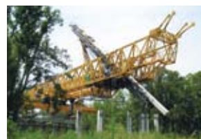
The pile is loaded into the lead with an attachment for the hammer clamped to its top. The lead then rotates the pile into a vertical position for driving.
