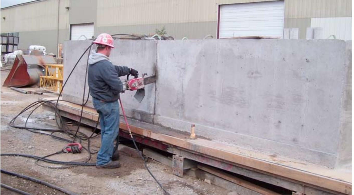
Concrete blocks were cut apart for examination of the duct coupler where installation procedures were tested in this mock-up of a precast segmental joint. Photo: Mn/DOT.
